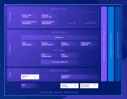
Figure 1: The openZDMs' platform Architecture
